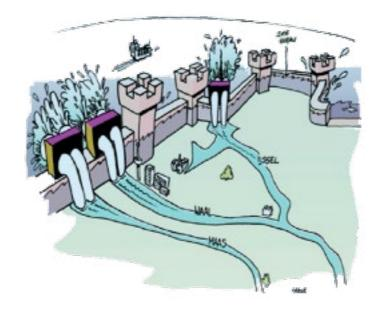
The '**protection-closed**' solution strategy involves reinforcement of the coast and closing-off of estuaries. In this case the rivers will no longer flow into the sea freely, and it will be necessary to pump river discharges into the sea. In addition, more room will be needed for temporary storage of river water. >
